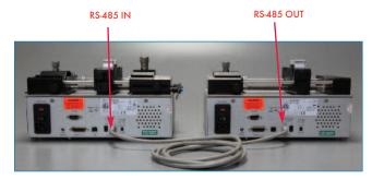
Plug in power cord to the Legato 210 (on the LHS) and connect the Legato 270 (RHS) to the Legato 210 using an RS-485 cable. Turn power switch on the Legato 210 to "on".
