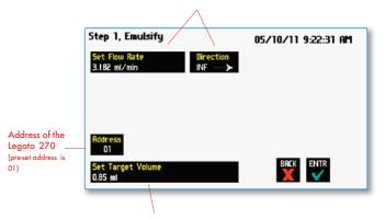
8. Set your target volume and then press the Enter button to return to the Step Definition screen. Select Step 2 to set the withdraw step parameters.
