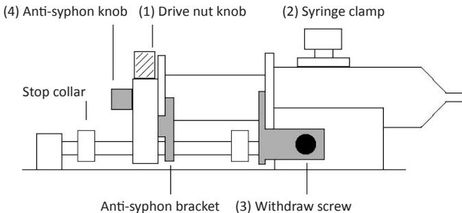
To simplify syringe loading, the pusher block can be disengaged from the leadscrew by turning the knob (1) and manually moved along the guide rods. Alternately, the **Fast forward, Fast reverse** feature can be used (press Run and respective Arrow key simultaneously).
