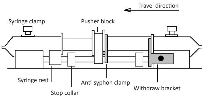
**Push-Pull operation:** Operate in Withdraw Mode.
