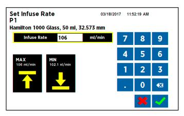
Set Rate Screen with MAX Flow Rate Selection
