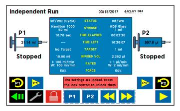
Independent Condition Run Screen Showing Locked Screen
