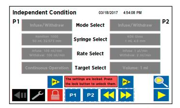
Independent Condition Setup Screen Showing Locked Screen
