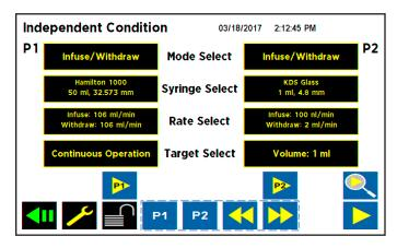
Setup Screen Showing Target Select "Continuous Operation"
