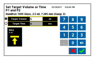
Twin Condition Target Select for x2 Gang Setting Showing 5 ml maximum volume
