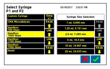
Twin Condition Syringe Select Screen (Showing Gang x1 and 2.5 ml Syringe Selection)
