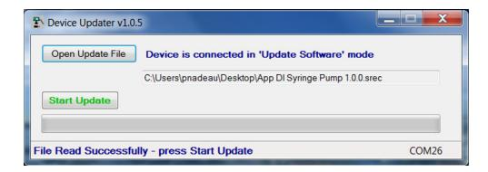
8. After the update is complete, press Reboot to power cycle the pump (see below).
