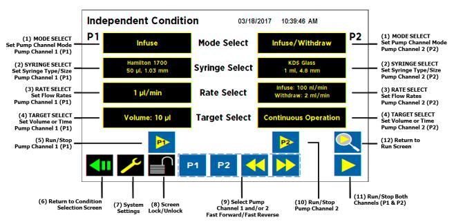
Independent Condition Setup Screen BUTTON Guide
