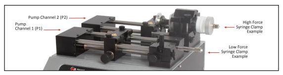
Syringe Pump Showing Syringes Installed with Low Force (P1) and High Force (P2) Syringe Clamps
