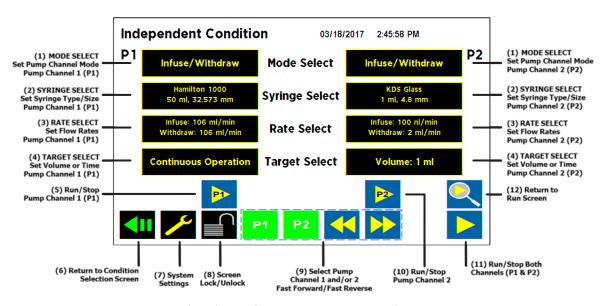
Independent Condition Setup Screen BUTTON Guide
