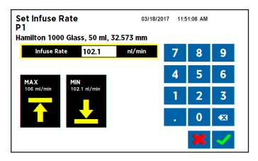
Set Rate Screen with MIN Flow Rate Selection
